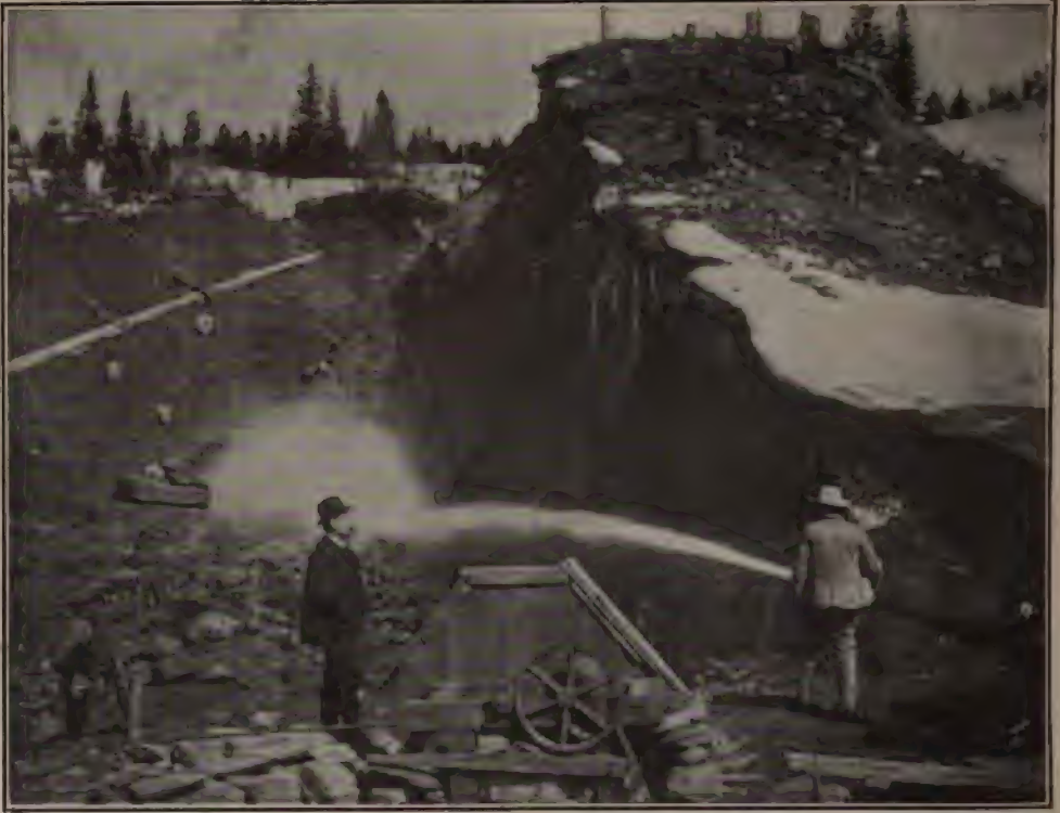
HYDRAULIC MINING IN THE MOUNTAINS OF PLEMAS COUNTY IS CARRYING THE MOUNTAINS DOWN TO THE SEA
